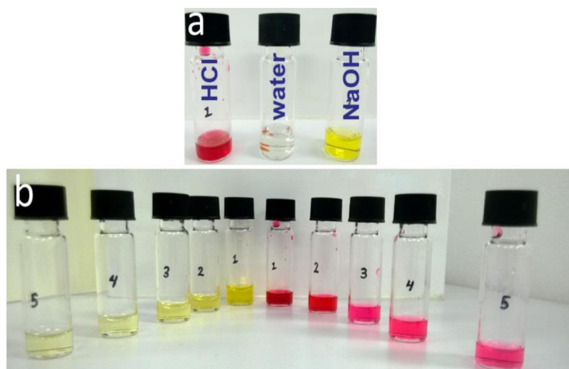
Figure 10. (a) Indicator (MR) release from the gel beads due to pH changes; (b) successive leaching showing that after 5 repetitions, leaching of MR was still observed.
